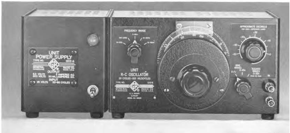
Figure 1. Panel view of the Type 1210-B Unit R-C Oscillator and the Type 1203-A Power Supply. The oscillator plugs into the power supply and can be secured to it with a bolt and butterfly nut to form a rigid assembly.
